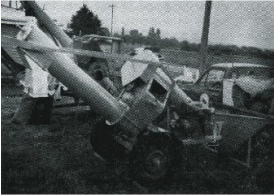
FIGURE 1. A Gibson carrot cutter. Carrots are dumped into the basket on the right of the photo, cut and poisoned in the middle chamber, and expelled through the screw conveyor on the left. The Urquhart prototype is in the background.
