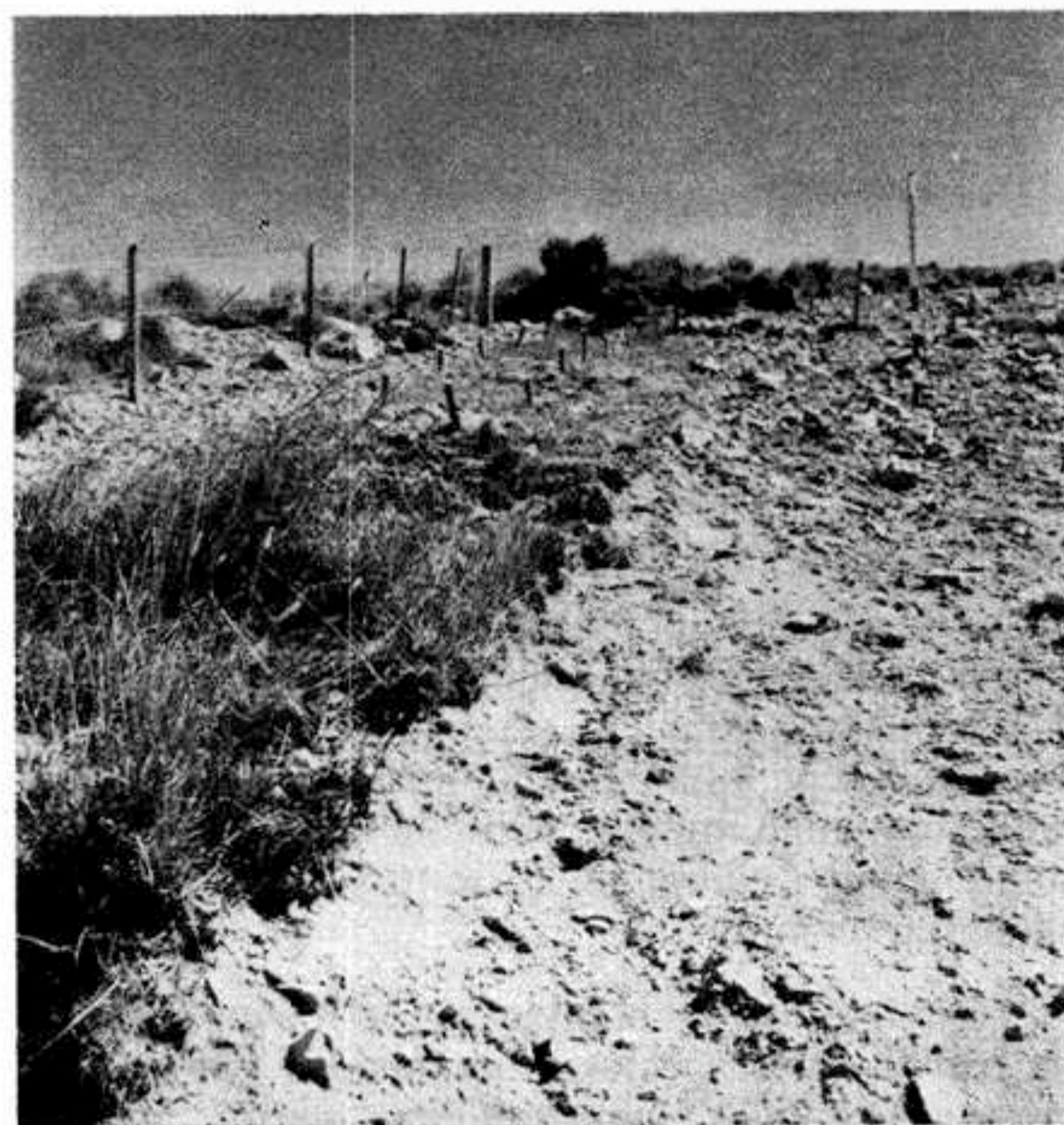
FIGURE 3. After five seasons the grass species sown with fertiliser are seen to have exerted a strong stabilising effect on subsoil on this slope.
