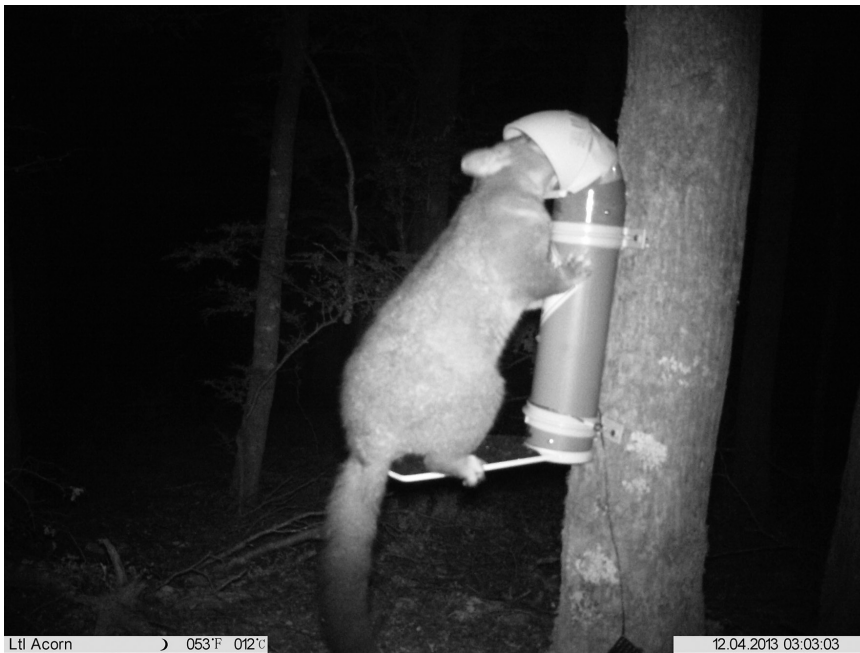
Figure 1 Brushtail possum, Trichosurus vulpecula , interacting with the resetting delivery system (RDS). The lower platform is a weight-activated trigger (set to >1 kg, but adjustable). The upper trigger has a long-life lure which must simultaneously be touched along with weight activation for the unit to dispense a measured dose of a zinc-phosphide gel.
