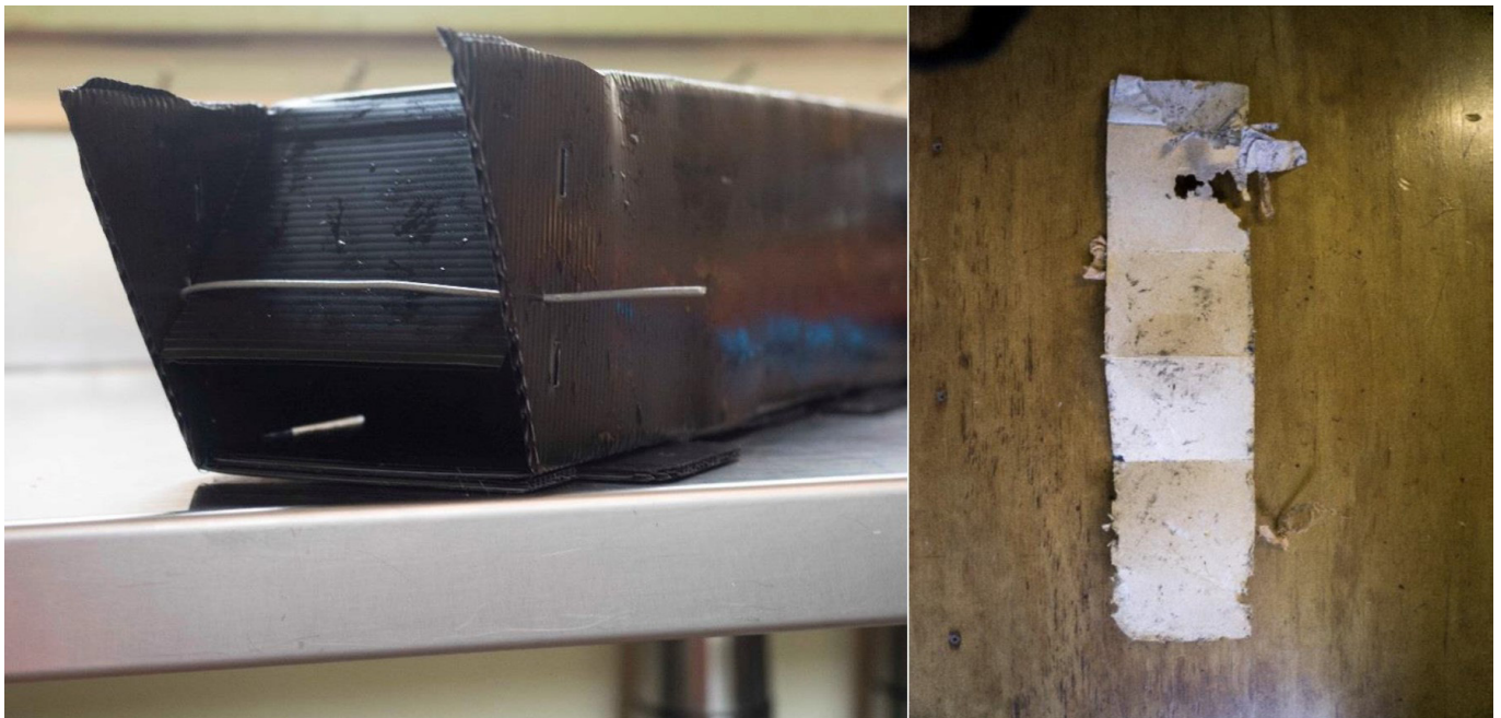
Figure 2. (A) Tracking tunnel with modified entrance (50 mm x 100 mm opening) to exclude birds; and (B) tracking card damaged by a parakeet (chewed edges).
